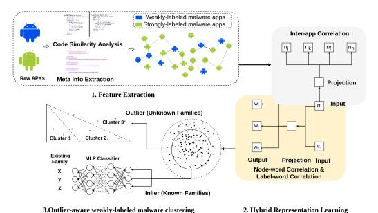
Fig. 3. The overview of ANDRE.  $n_i$  represents a single malicious app, and  $c_i$  denotes a known family name if  $n_i$  is a strongly-labeled.  $c_i$  is empty if  $n_i$  is weakly-labeled for prediction purposes.  $w_i$  denotes a word in the meta-info associated with a node.
