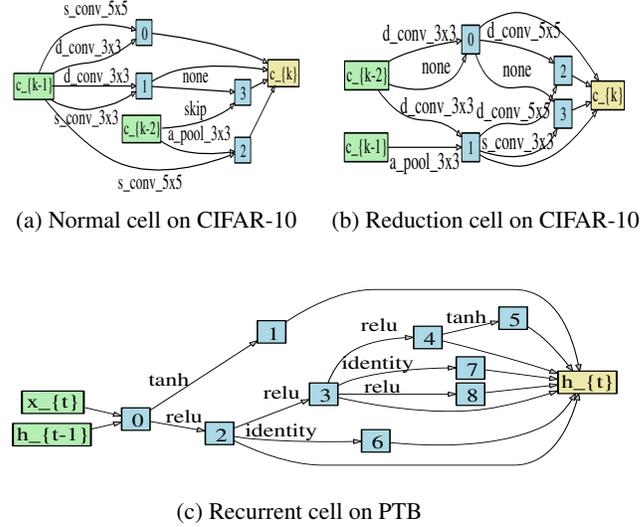
Figure 1: Best cell structures found by our algorithm. For CNN cells, each node needs to select two former nodes with applied operations as its input. As to RNN cells, each node only selects one former node with applied operation as its input. The outputs for the three types of cells are the summation of outputs for all nodes.
